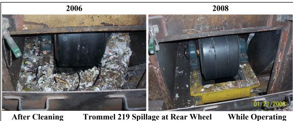
**After Cleaning Trommel 219 Spillage at Rear Wheel**
