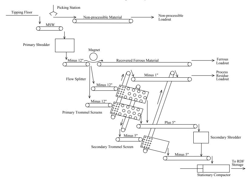
In addition to operating the equipment during processing hours, the operating staff is responsible for cleaning the equipment after processing has ended. If the spillage is cleaned each day, it will not cause undue harm to the equipment. The maintenance staff is responsible for fixing the cause of the problem. In this example case, it would involve replacing or readjusting the skirting. This type of problem is easily controllable if good operating and maintenance practices are followed.
